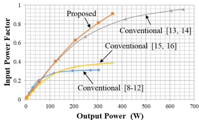
FIGURE 7. Simulated input power factor in the conversion ratio of 1/4
