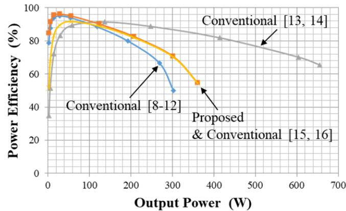
FIGURE 6. Simulated power efficiency in the conversion ratio of 1/4
