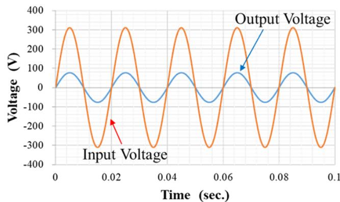
FIGURE 5. Simulated output voltage in the conversion ratio of 1/4
