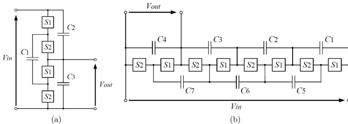
FIGURE 1. Conventional SC AC-AC converters: (a) basic converter realizing  $1/2\times$  step-down conversion [8-10] and (b) expanded converter realizing  $1/4\times$  step-down conversion [12]
