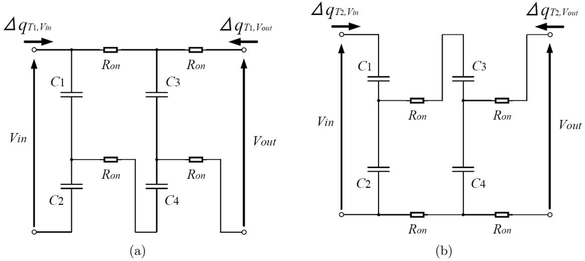
FIGURE 4. Instantaneous equivalent circuit in the conversion ratio of 1/4: (a) state- $T_1$  and (b) state- $T_2$
