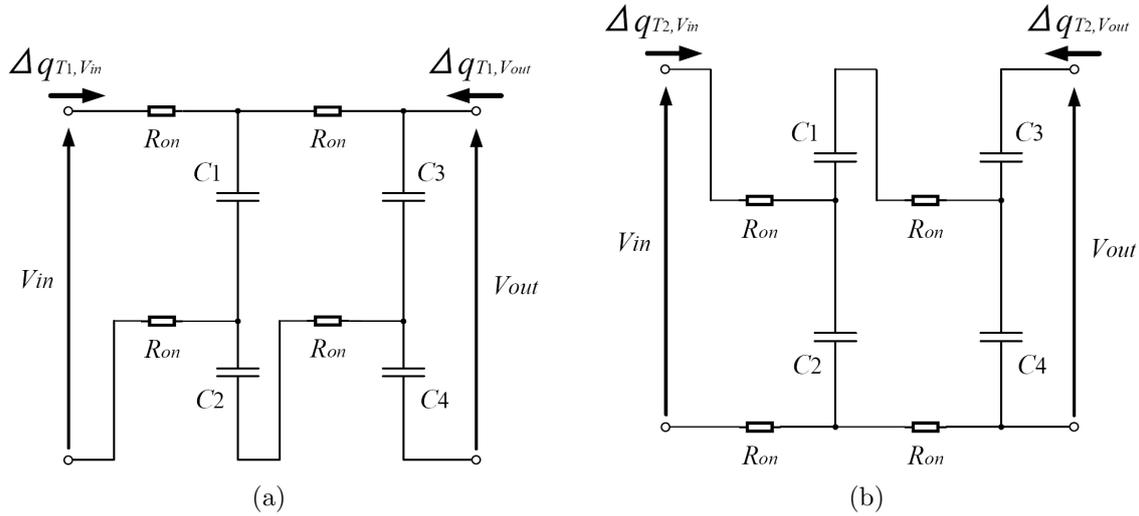
FIGURE 8. Instantaneous equivalent circuit in the conversion ratio of 4: (a) state- $T_1$  and (b) state- $T_2$
