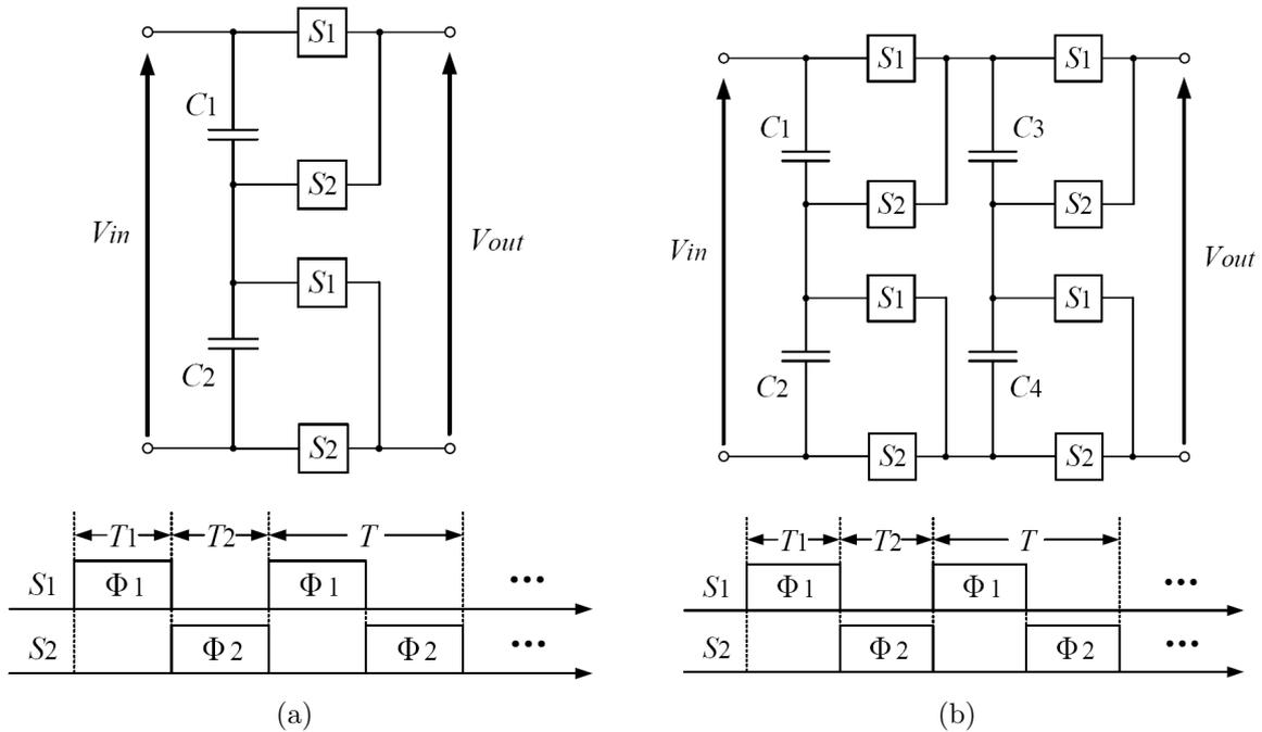
FIGURE 2. Proposed AC-AC converter: (a) basic converter realizing  $1/2 \times$  step-down conversion and (b) cascaded converter realizing  $1/4 \times$  step-down conversion
